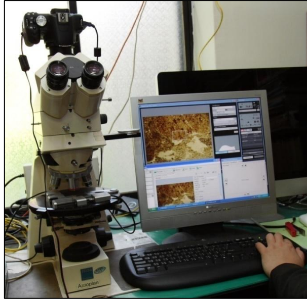
Figure 5.19: A binocular polarising optical microscope is connected with a computer system that allows photomicrographs to be digitally displayed on the screen.
