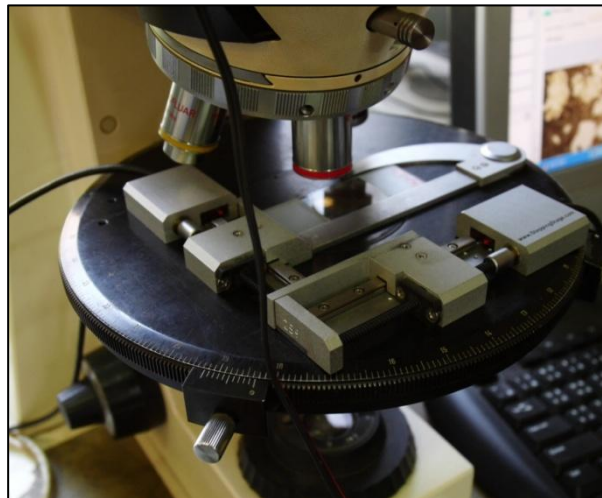
Figure 5.18: The stage with an attachment that allows the thin-section to be moved in fixed increments.
